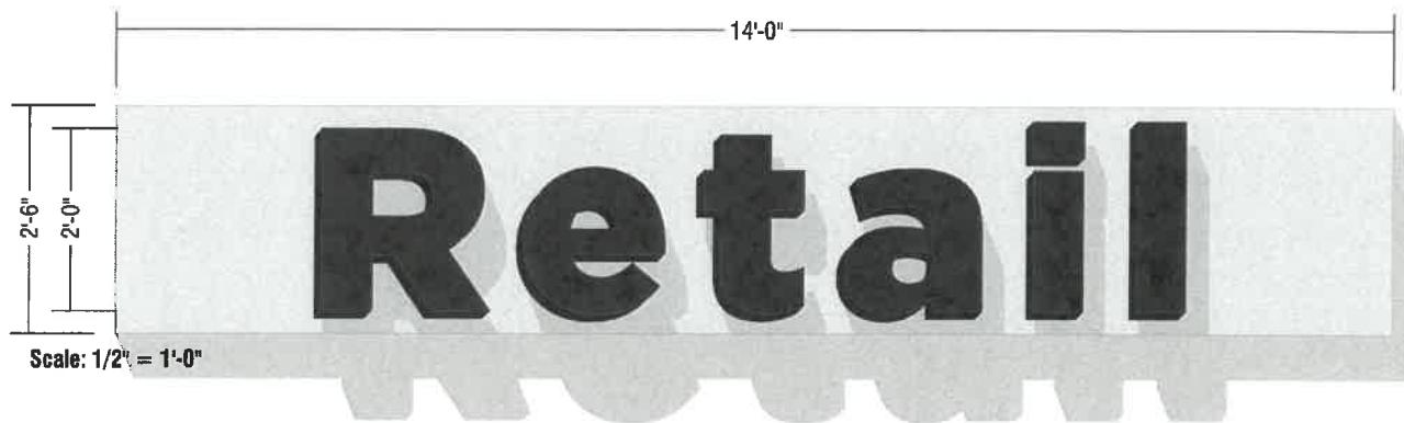
Reverse-Channel Halo Lighted Letters constructed of aluminum (2" deep). Halo illumination via LEDs. 120 Volts. All wiring UL approved. Letters mounted to aluminum sign pan (2½" deep) via 1½" stand-off spacers with non-corrosive fasteners.
