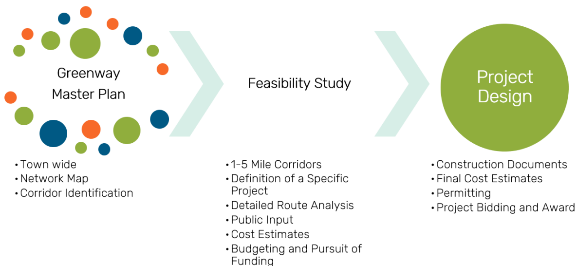
Figure 24- Greenway trail planning, design, and construction process and sequencing.
